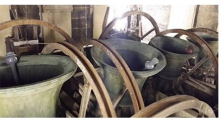
preparing the Ellecombe chiming system which allows one or two people to operate the bells, all be it at a reduced volume. We are fortunate to have this facility and it also allows us to ring tunes.
